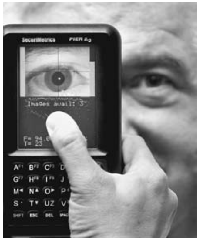
A portable iris recognition scanner being demonstrated at the Biometrics 2004 exhibition and conference in London. (IAN WALDIE/GETTY IMAGES)
