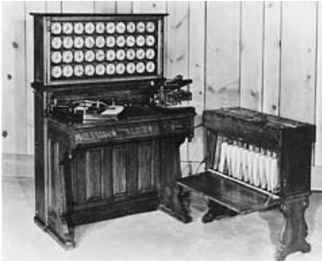
The Hollerith tabulator and sorter box, invented by Herman Hollerith and used in the 1890 U.S. census. It “read” cards by passing them through electrical contacts. (HULTON ARCHIVE / GETTY IMAGES)
